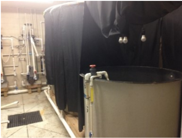
Figure 2. Recirculating systems for medium-scale larval rearing production (1-m 3 working volume per tank)
