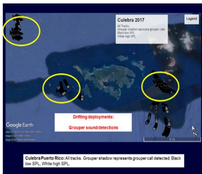
Figure 2. Sound-drifter tracks overlaid on map of Culebra. Black circles represent low sound pressure levels, white circles represent high sound pressure levels, and grouper shadow icons represent distinct grouper calls. Yellow ovals highlight drifter deployments where red hind CAS sounds were detected in winter 2017. Tracks to the SE represent summer 2016 deployment when Haemulid fish chorusing was recorded.
