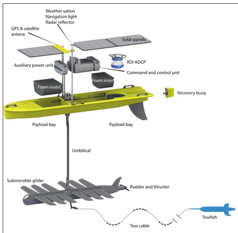
Figure 2. Components of the SV3 wave glider.
