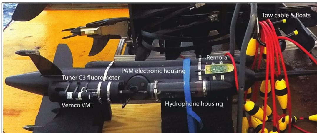
Figure 3. Components of the tow-body.
