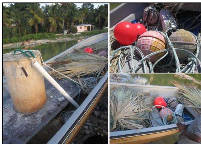
Figure 2. Photographs of different components of a low cost FAD unit about to be deployed in Port Salut, South department, Haiti. The left panel shows the mooring component, a drum filled with concrete and miscellaneous metal elements; the top right panel shows several units of two types of buoys (used for the floating component) attached to a polypropylene main line and cable wire (the latter usually follows the main line for the first 50 meters); the bottom right panel shows the surface aggregator made up of palm leaves. Further details can be found in Vallès (2015). All photographs taken by H. Vallès.
