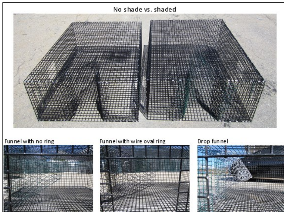
Figure 4. Experimental design. Treatment level 1: No shade vs. Shaded; Treatment level 2: funnel variations.
