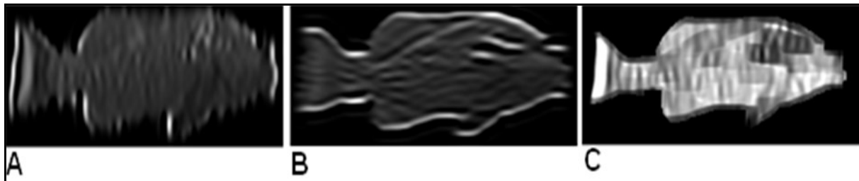
Figure 4. Filtering results of horizontal and vertical Gabor filters on EM. A. Filtering result of horizontal Gabor filter. B. Filtering result of vertical Gabor filter. C. Ratio image.
