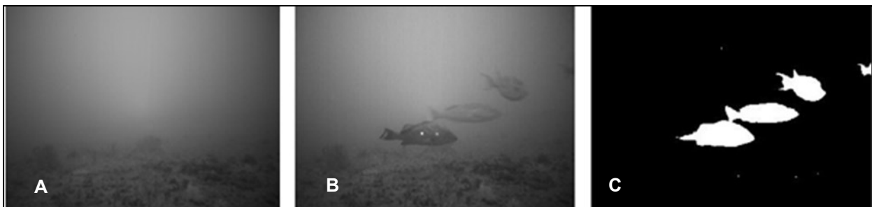
Figure 1. Background Processing Steps: (a) Background image, (b) an original frame, (c) thresholded frame
