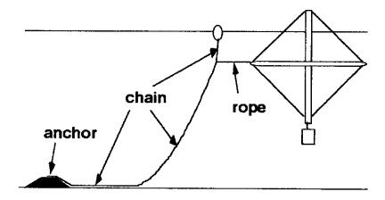
Figure 2. Representation of the Gulf of Mexico Offshore Aquaculture Consortium single-point mooring (SPM) system and Ocean Spar Sea Station cage.
