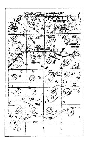
**Figure 1.** Area surveyed with SSS off La Parguera, southwest coast of Puerto Rico. Area extends from shore to shelf edge. Each square has 1 nm². Right most column was not included in the survey.
