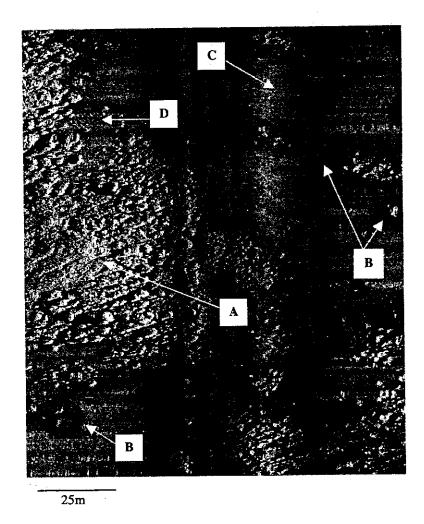
Figure 2. Edited single SSS image from 17'56'N, 67'03'W with water column removed. Surface echo has been edited out for easy interpretation. A. Strong rugose reflection shows coral reef habitat. B. Patch surrouned by halo of dense halophila decipiens. C. Smooth sand and algae plain. D. Sand ripple ridges.
