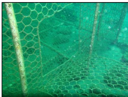
Figure 6. Opened escape panel.
