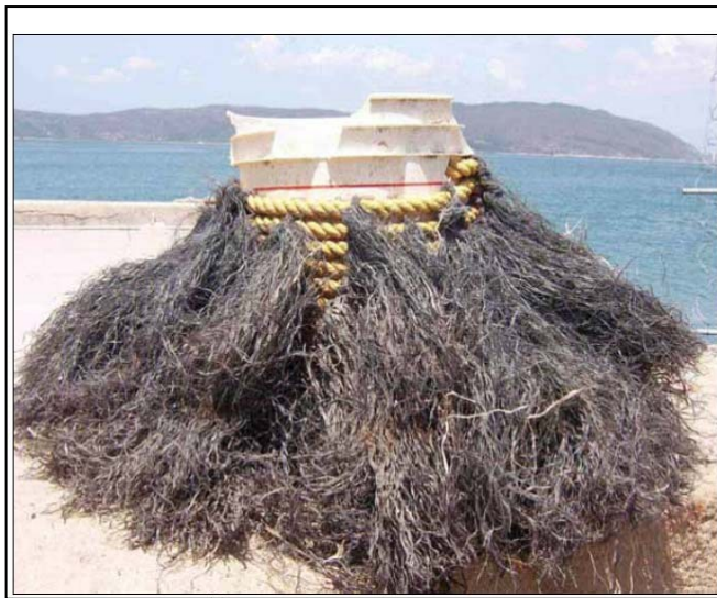
Plate 1. Modified GUSI lobster postlarval collector used in present study with central plastic bucket and teased-out black synthetic rope tassels forming "skirt" around bucket.
