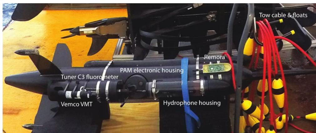
**Figure 2.** Components and payload of the tow-body.
