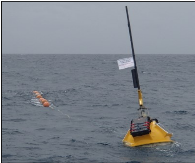
Figure 11. FAD equipped with acoustic material to register earthquakes around Guadeloupe (OVSG).
