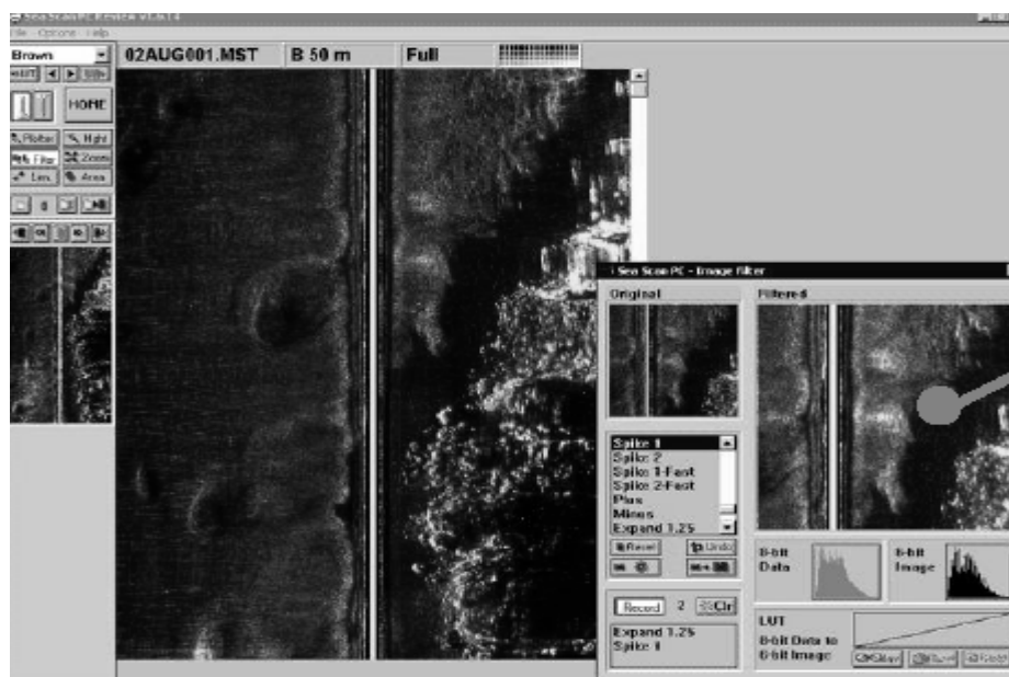
Figure 2. Picture illustrating acquisition of SSS images when using the 300 kHz Marine Sonic Technology system.
