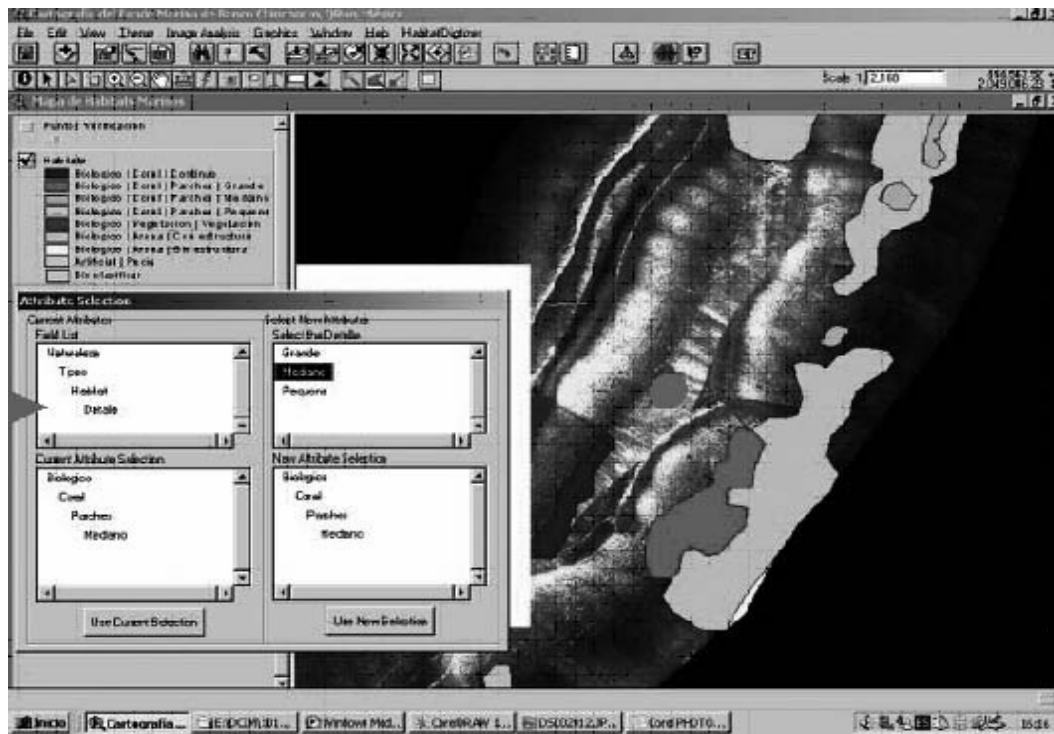
Figure 3. Example of habitat mapping being digitized from the Geotiff habitat mosaics using the habitat digitizer extension developed by NOAA/NOS/Biogeography Team in Arc View GIS 3.2.
