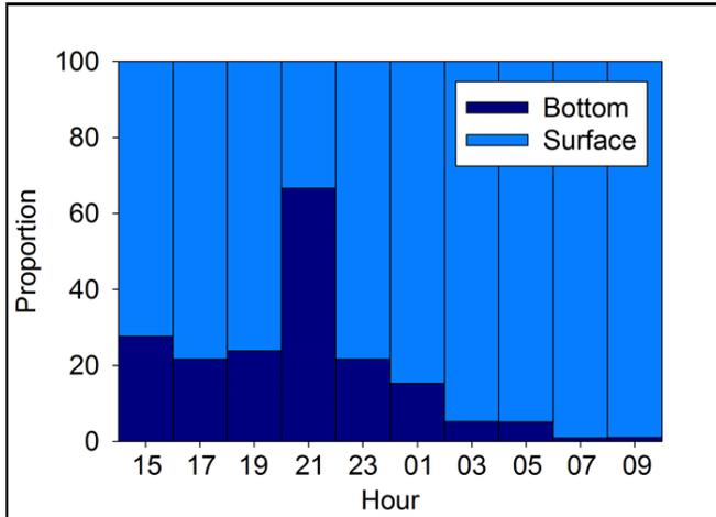
**Figure 3.** Proportion of fish abundance distributed in upper (surface) or lower half (bottom) of the water column, observed from orthogonally rotated (vertical) sonar averaged over a period of interest throughout the 70 hour deployment.
