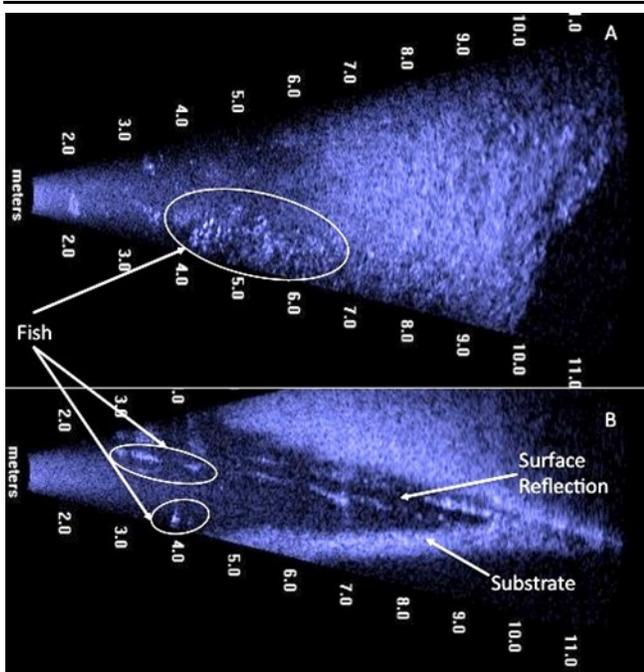
**Figure 1.** Example of horizontal (A; lateral) and vertical (B) rotation of the DIDSON sonar deployed at the confluence of the subtidal-intertidal system. The lateral view shows the extent of the tidal channel at approximately 10 m in range from the sonar. The orthogonal view (B) illustrates the vertical perspective with the reflective water surface and substrate interfacing at approximately 10 m range to the sonar.
